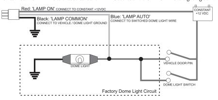
For **NEGATIVE SWITCHED** Systems connect the BLUE wire to the vehicle's dome light switched wire. Then connect the BLACK wire to a fused constant +12VDC source and the RED wire to a good ground.
